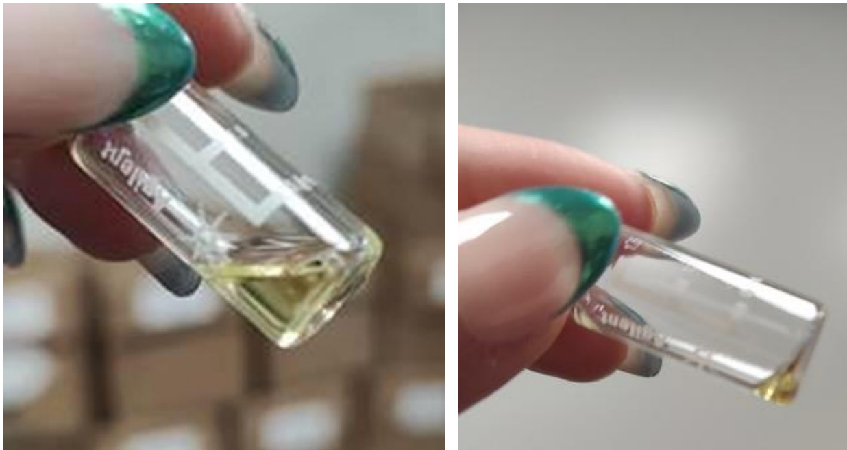
Figure 1 - Condensate recovered from flashed downhole reservoir fluid samples from Mukuyu-2 / ST-1 well from Upper Angwa (on left) and Lower Angwa formations (on right) with API gravity of 50-60
