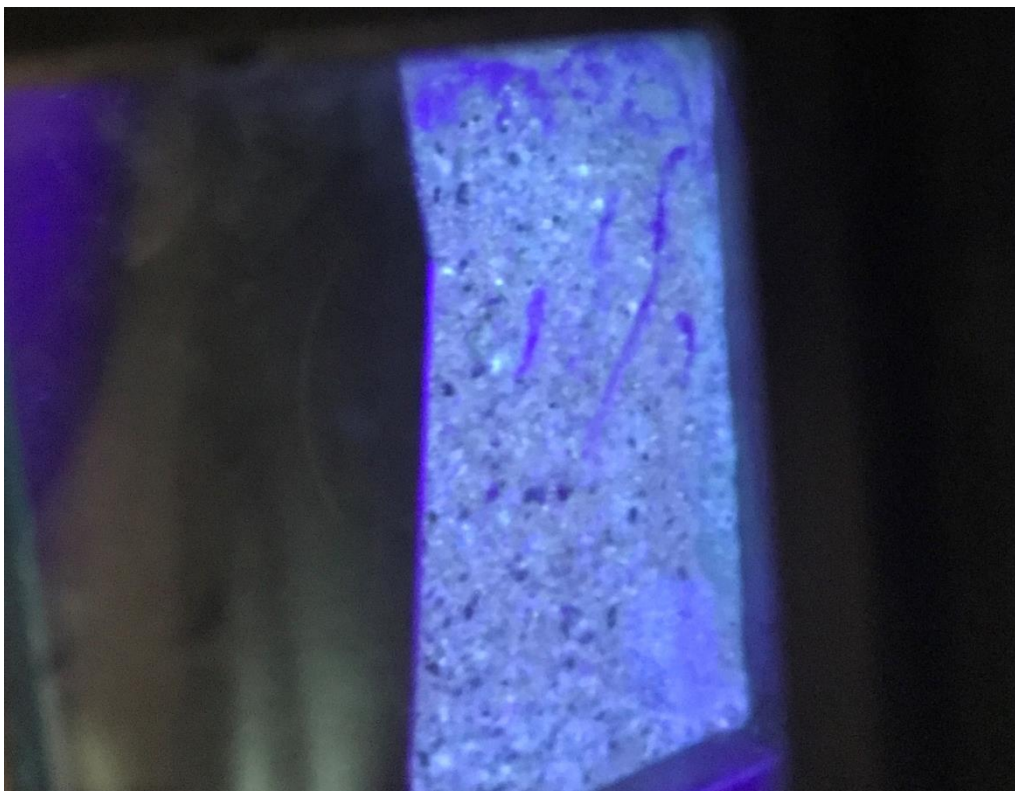
Figure 1 - Fluorescence in cuttings from Lower Angwa reservoir @ 3,645mMD with associated gas shows and drilling break
