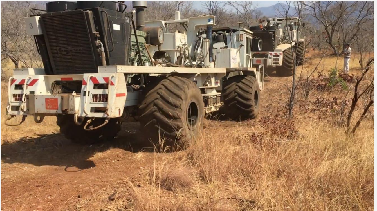
Figure 1- Vibroseis units in the field acquiring data during the CB21 Seismic Survey
